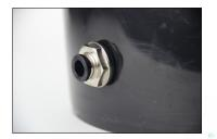
5. Once you install the reservoir bulkhead it will look like the photo. Plug in a piece of tubing or a plug into the newly installed reservoir bulkhead. Test for leaks by filling up the container with water and leaving it for 30min. The connection should be completely water tight.
