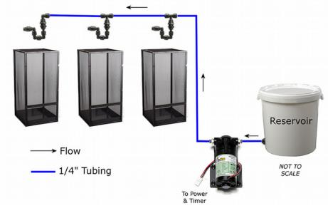
Systems that do not have a ZipDrip valve connected, terminate with a final elbow misting assembly or a T-misting assembly that has been plugged. Whether you are connecting a single or multiple nozzles, the idea will be the same. For illustration purposes, we are showing an install with 3 nozzles.
