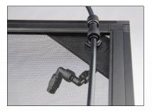
Plug in the included fitting and push in the tubing to finish the misting assembly install. You can connect multiple assemblies together as needed. Remember to push the tubing in all the way so it passes the rubber oring inside the fitting. If the connection leaks, simply push it harder to ensure a proper seal.
